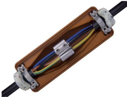
PVM...EG, PVS...EG Cast resin straight-through joint with integrated strain relief, for polymeric cables and conductors, with cast resin EG
