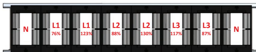
Non-Optimized Conductor Arrangement (Load current unbalanced)
