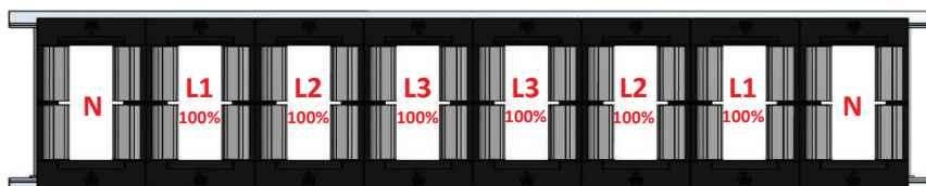
Optimized Conductor Arrangement (Load current balanced)
